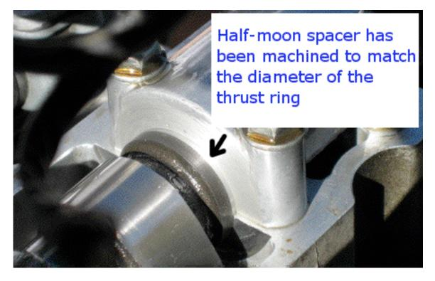
This photo shows a half-moon spacer controlling the endfloat through the bearing cap.
