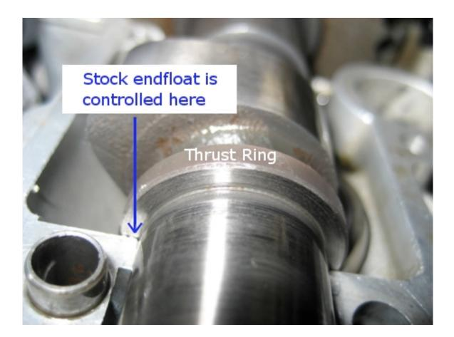
I measured the gap between the thrust rings and the bearing thrust faces. The inlet cam thrust clearance was 0.005 in, the exhaust was 0.006 in. I calculated that the stock clearances should have been 0.0015 in for each camshaft.
