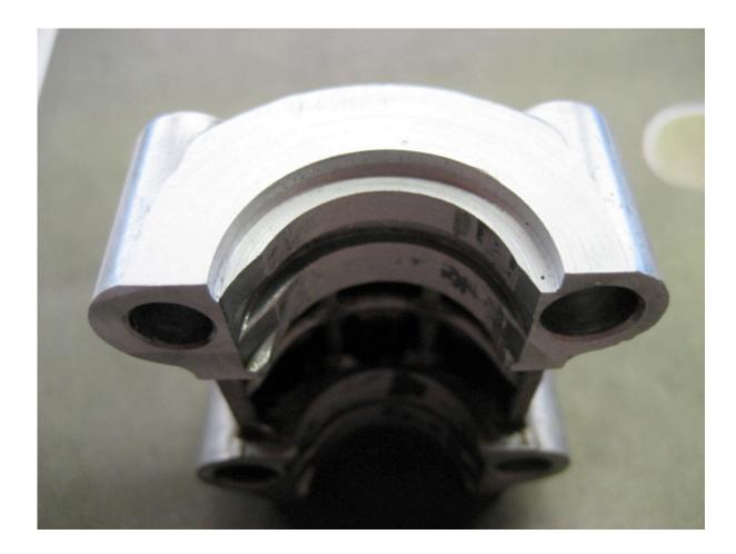
This photo shows a bearing cap after the spacer recess has been machined. Note the slight radius left in the corner of the recess. Thrust spacers are machined with a chamfer to accommodate this fit-up.
